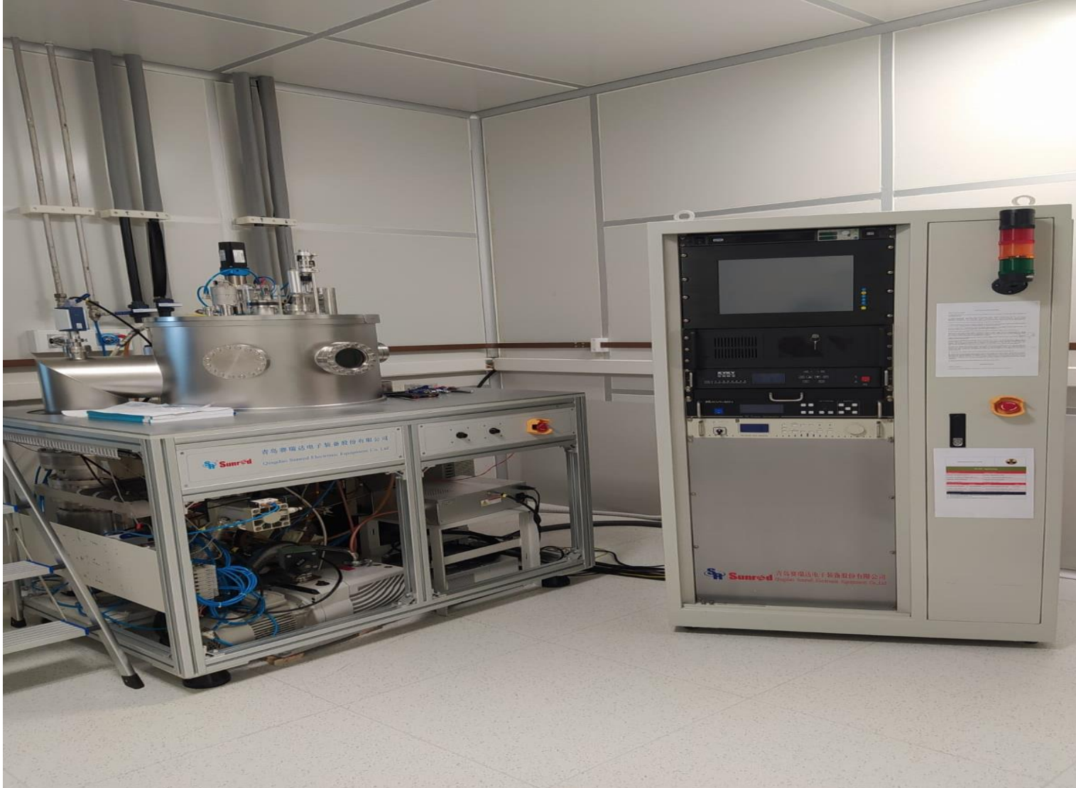
The sputter machine from which the Aluminum contacts were deposited
